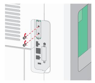
**c** Insert the plug of the printer hard disk interface cable into the receptacle of the system board.
