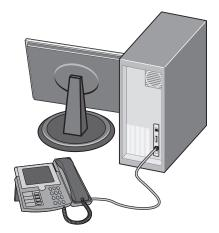
**5** Connect a third telephone cord from the computer modem to the EXT port of the printer.
