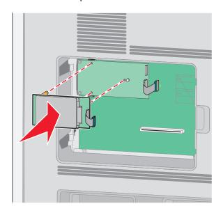
**c** Insert the plug of the printer hard disk interface cable into the receptacle of the ISP.
