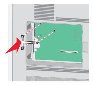
**6** Install the ISP onto the plastic tee. Angle the ISP over the plastic tee, and then approach the plastic tee so that any overhanging connectors will pass through the ISP opening in the system board cage.
