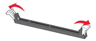
**4** Align the notches on the memory card with the ridges on the connector.
