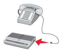
**5** Connect a third telephone cord from the answering machine to the EXT port  $\widehat{\underline{\ }}$  of the printer.
